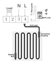
For the correct connection of the Webtech mat, please, pay attention to the colours of the installation wires. The blue and brown/black (live) installation wires are connected to the thermostat. The earth wire must be connected to the earth.
