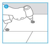
Boards are fixed to timber floors using an adhesive plus screw and washer method. The following procedures must be observed:
