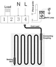
For the correct connection of the Webtech Elite mat, please, pay attention to the colours of the installation wires. The installation wires are connected to the thermostat. The earth wire must be connected to the earth.
