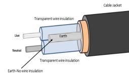
*Note:* On mat sizes 2.0m2 and above the Live and Neutral wires are interchangeable
