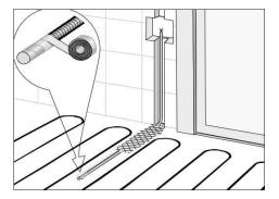
3. Place the cold cable in the appropriate channel.
